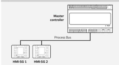
The controller can be installed using a wall wiring box or embedded in plaster. The maximum distance between the control unit and room controller is up to 700 m. HMI-SG controllers are connected to the master controller in series and wiring is always performed to one point.
