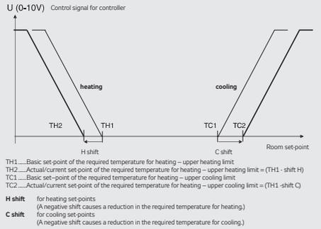
**Figure 13 – Set-Point Compensation (Shift) Description and Settings**
